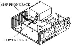
3). Connect the DB-9 connector to the computer's serial COM port. Connect the 4P phone plug connector to the added I/O bracket. See below illustration.
